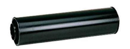
A silencer is essential in every central vacuum unit. It should be installed on the air expulsion pipe, near the grille: the type of silencer is chosen based on the diameter (Ø) of the expulsion pipe. A silencer with a diameter larger than the outlet diameter of the central vacuum unit is recommended for expulsion lines longer than 6 metres.
